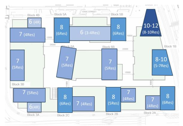
Fig 5.4: Proposed Site Layout Concept - Building Heights (Illustrative Only) (Assumes that Ground Floor Retail/ Commercial (6-7 metres) is equivalent to 2 floors)
