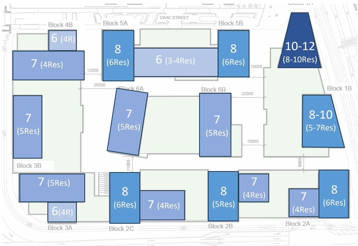
**Fig 5.4: Proposed Site Layout Concept - Building Heights (Illustrative Only)**
